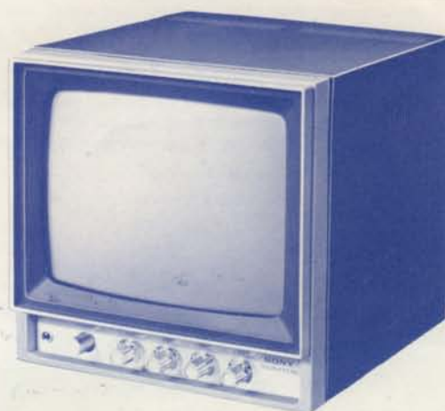
Compact, lightweight 9-inch monitor with DC clamper High resolution, video only
